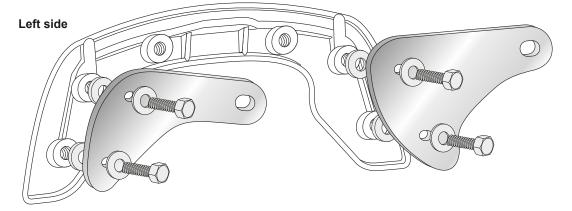
Fix the C-Bow with mounted adapters at the chrome bar of the bike. Use allen screws M10 x 90 x 1,25 with washer ø10,5. Sandwich spacer ø18 x 11 x 40mm.
