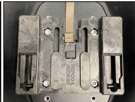
Disassemble the locking unit.
