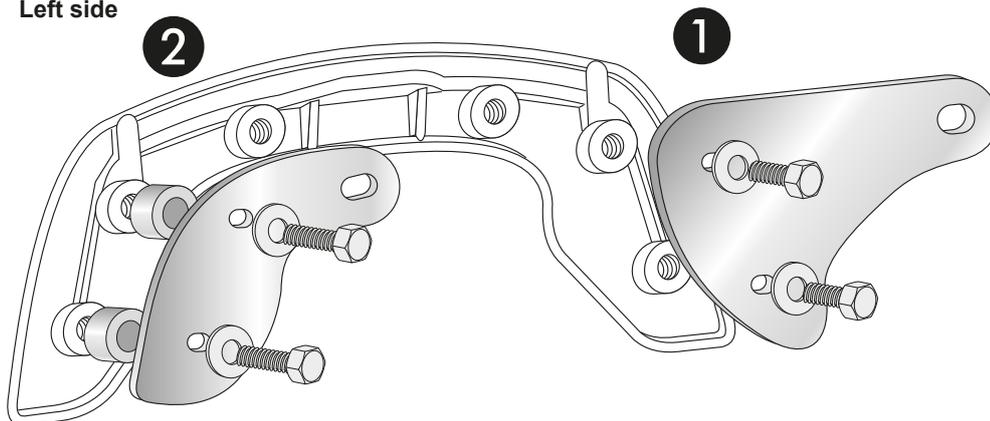
**2** Fix the C-Bow with mounted adapters at the chrome bar of the bike.
