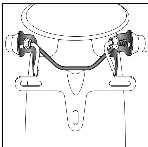
Position the blinker mounting so, that the round steel bar number lays on the plate holder.
