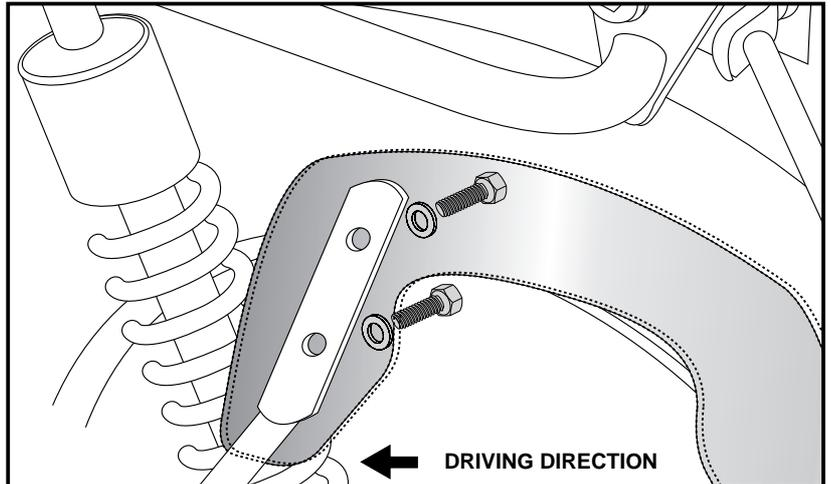
**4** Fastening of the C-Bow to the rear adapters left + right:
