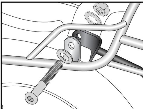
When mounting a C-Bow together with a Sissybar/a rear rack, the C-Bow will be placed between frame and Sissybar.
